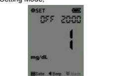
press Up and Down button to switch clock, press Home button to edit the selected clock;
