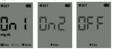
Press Up and Down button to switch, press Home button to confirm and enter into next setting item;
